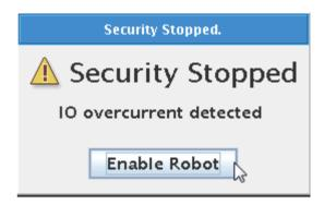
The output is not current limited, but if the output is short circuited it will result in a security stop and error messages because of over current detected on an output.
