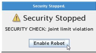
If you turn the joints all the way and beyond its limitation you we will se an Error messages "Joint Limit Violation" which is a safety stop in order not to spoil the inside of the joint. Press "Enable Robot" to acknowledge the error messages.
