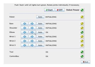
After a few seconds the "Elbow" joint will report "OK" on the monitor. This means the robot now knows where this joint is positioned. It is not necessary to turn one full circle. What you see on the photo is normal.
