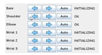
After a few seconds the "Shoulder" joint will also report "OK" and the position of the joint is now know to the robot controller.
