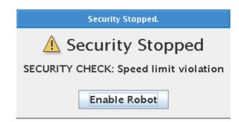
The robot started to move from Waypoint\_1 towards Waypoint\_2 in a straight line, but when the physics was in the way the robot showed the phenomena about increasing in speed and then rapid security stopped with "Speed limit violation" and never reaches Waypoint\_2.
