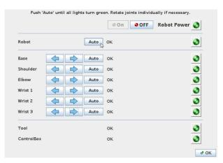
Keep pressing the "Auto" button. Now notice how the remaining 4 joints all move until all of them say "OK" which means the robot has been Initialized and all joint position are know to the controller.
