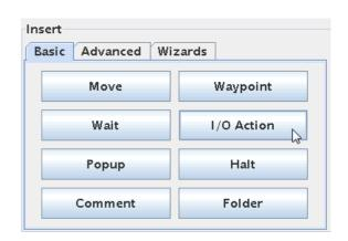
Since we already have to program lines then we need to decide where we want to have out action. In this case we want it in between the two Waypoints so we place the cursor by pressing the first Waypoint. Press the "Structure" tab. This time choose an "I/O Action".
