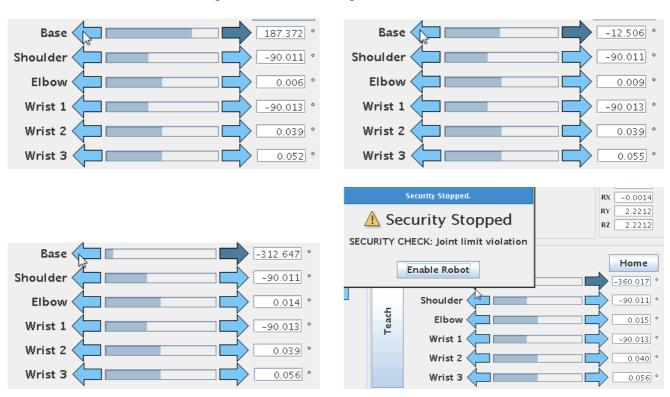
The same error messages occur when you turn the robot joint 720 degrees all the way to the other side. Press "Enable Robot" to acknowledge the error messages.
