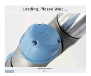
During boot you will see various screens loading and checks – this is normal and it takes 1 – 2 minutes to boot. You will also hear the fans turn in the controller box.
