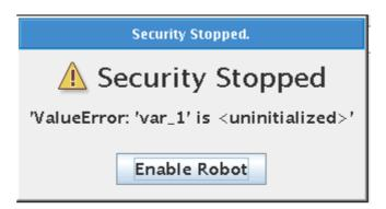
If you get this error messages it is because we need to tell the Robot – what should the variable "var\_1" be when we start the program. This is uncertain for the robot if we have not explicit set the variable before the program execution.
