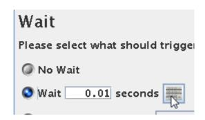
In this case we want to have a flat Wait based on time for 2 seconds. Tick the "Wait 0.01 seconds" tab. Press the "Keyboard" symbol in order to define the Wait time.
