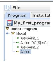
Continue programming we wish to control the same output after the robot has moved to the Waypoint\_2. Press the Waypoint\_2 and go to "Structure" tab and pick one more I/O action.
