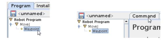
We need to define each Waypoint we insert into out program. Point and press on the Waypoint we want to define – in this case there is only one because we just started programming. Press the "Command" tab.
