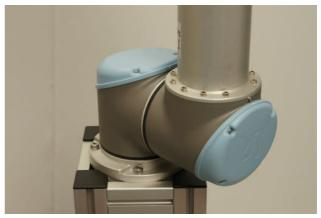
Now the robot is fully stretched is a nice position to start moving each joint to see how the robot moves. Start with the base joint and press the Arrow bar left or right and see how only the base joint moves.
