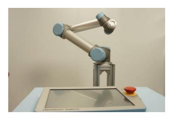
All the joints on the monitor reports "OK" and notice how all the lamps turned green. The robot is now initialized and ready to be programmed or load a program if we already have made a program before.
