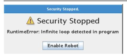
If you get this error messages is because the robot does not like to be caught in an Infinite loop. In this case the Thread program might be Infinite if the "var\_1" never change.
