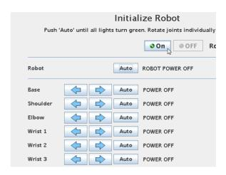
Press the "ON" button to turn on the power to the robot.
