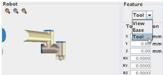
In the middle of the move screen is a graphic representation of the robot position which is useful as a guide for the robot posture. You can choose between two different views (Base view or Tool view) i.e. angles of the graphic representation.
