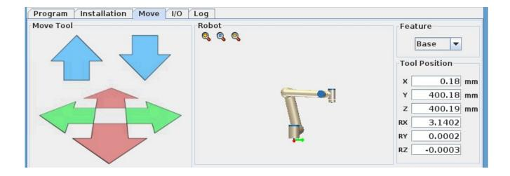
Notice where the cable is coming out from the robot in the Y axis. Joystick movement is from the base in Y direction.
